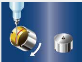
Dispensing of 2-part epoxy adhesive to motors
