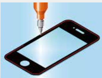
Sealant dispensing of PUR for smartphone's cover
